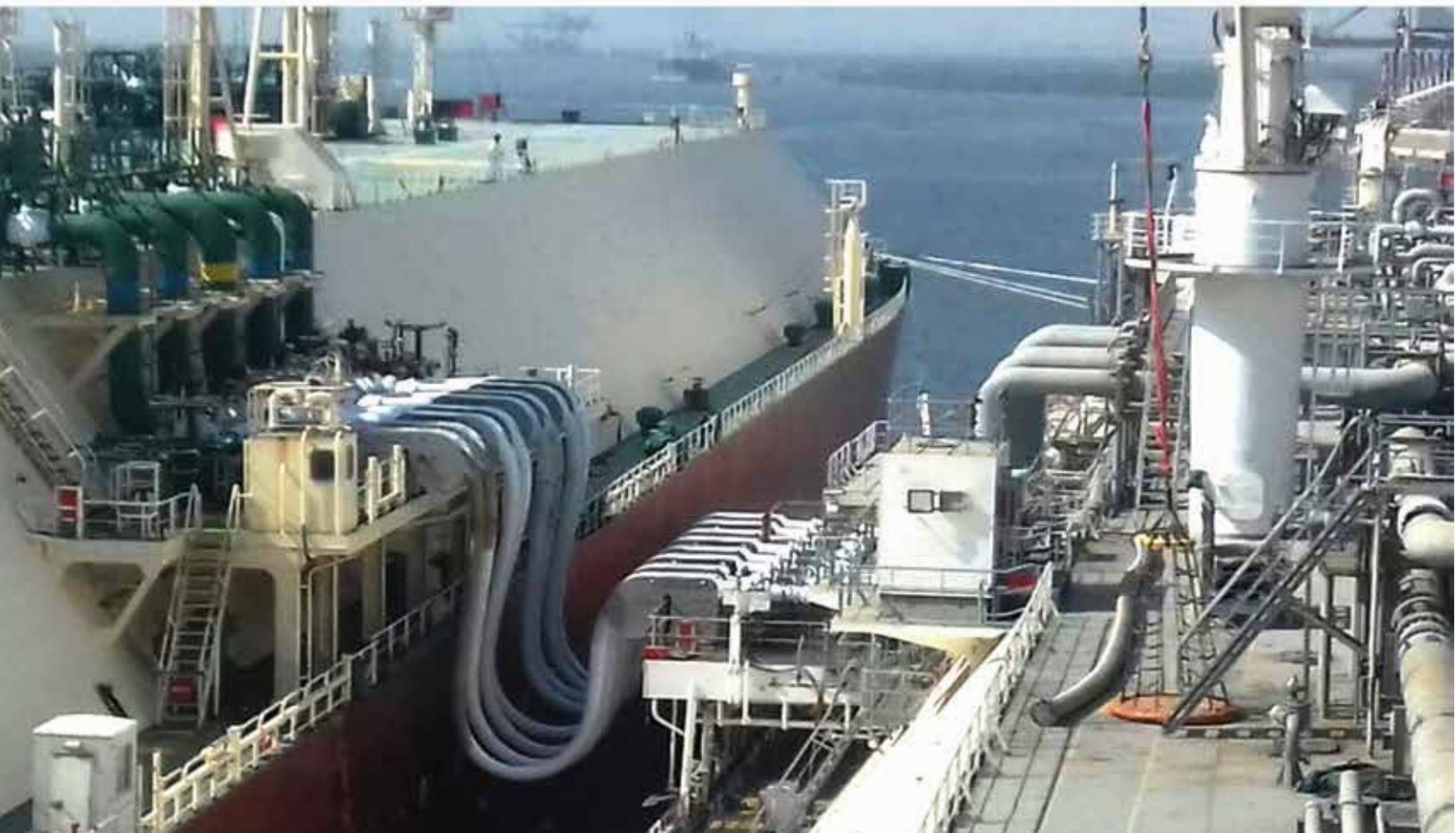
Mitigating shortfall: Ship-to-Ship transfer of LNG underway at Elengy Terminal Pakistan Ltd.
